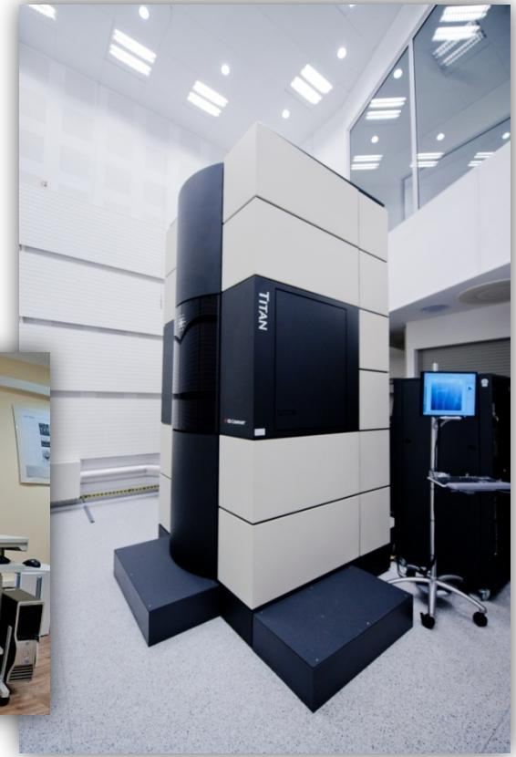
The latest generation analytical electron microscope (S)TEM FEI Titan Cubed G-2 60-300
